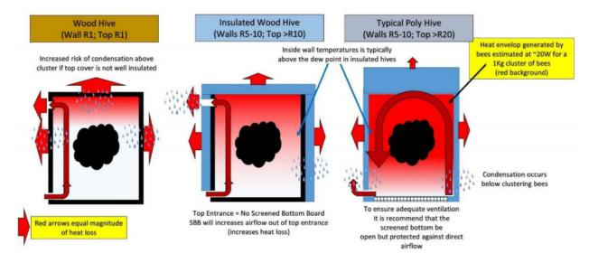
Figure 3. How Insulation Works (Tardif, 2020).
